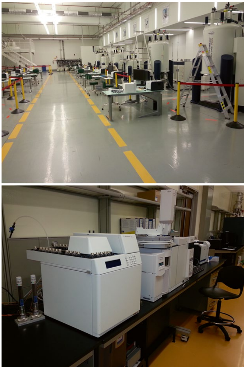
Fig. 2 Typical NMR laboratory (KAUST NMR laboratory) where sufficient, separated space is required for location of NMR spectrometer ( top ); GC-MS where the GC-MS is usually small enough to be allocated on lab bench top ( bottom )
